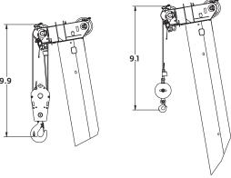
Dimensions are for the largest grove furnished hook block and overhaul ball, with anti-two block activated.
