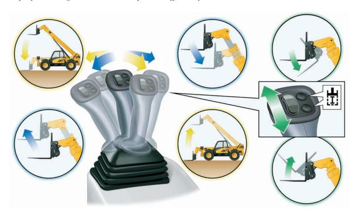
**Joystick Control.** The joystick allows three simultaneous boom functions and incorporates a unique slider switch.
